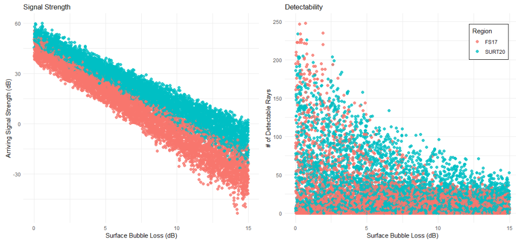
Figure 5.7: Raw model outputs plotting signal strength (dB) and detectable rays versus surface bubble loss (SBL, dB), separated by scenario.
